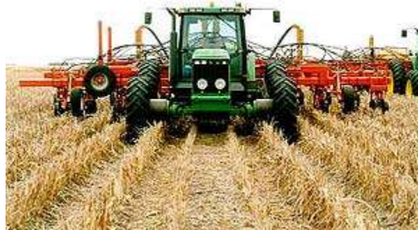
Figure 2 Modified tractor used in controlled traffic farming
