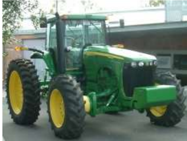
Remove inside duals to leave outer wheels on 3m track
