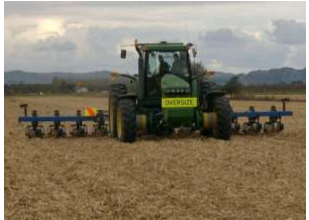
The 12 row strip-till machine prepares strips in autumn with soil in optimum condition
