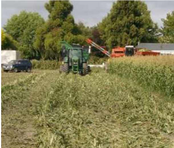
Harvester, tractor and gondola all driving on different lines, compacting the soil
