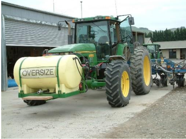
Tractors have RTK-GPS and auto-steer
