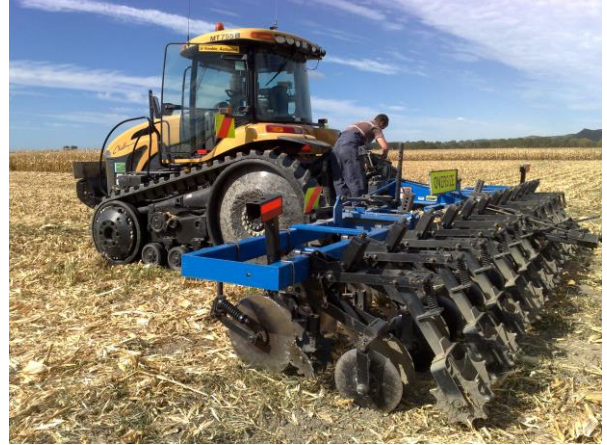
The 12 row strip-till machine prepares strips in autumn with soil in optimum condition
