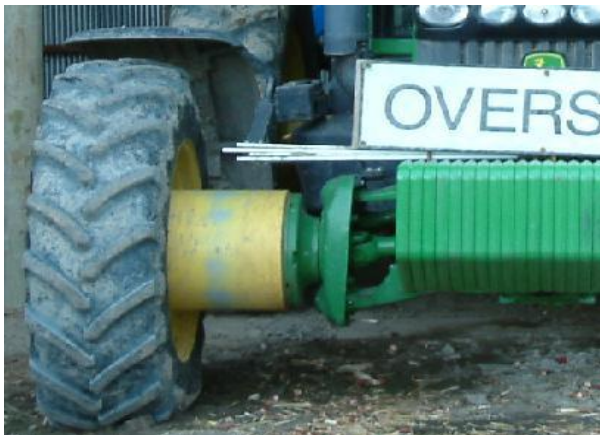
Cotton reel spacer extending front wheel track
