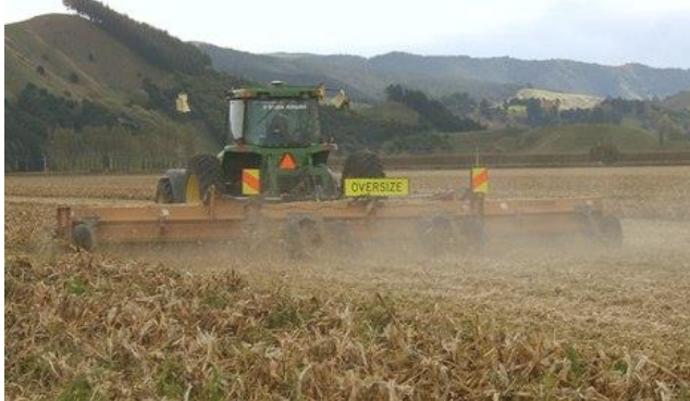
The triple flail mulcher unit covers 9m at a pass
