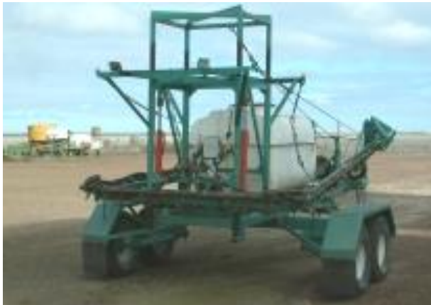
Trailed sprayer built with 3m track
