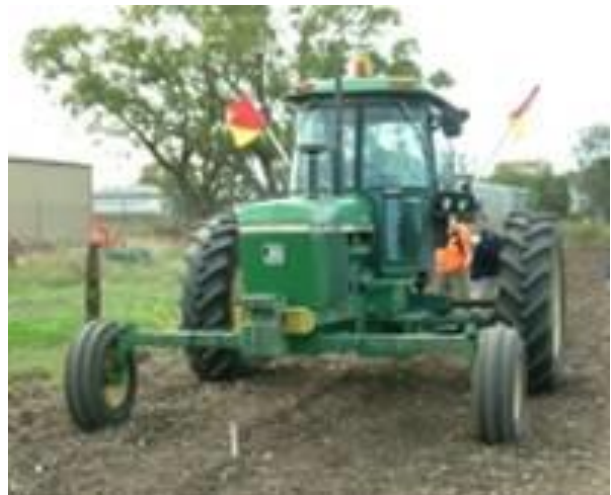
Front axles can be easily widened on 2WD machines
