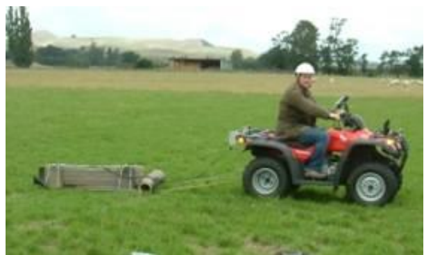
EM38 Soil scanner mapping soil variability
