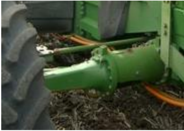
Axle extension to move front wheel centres out to 3m.
