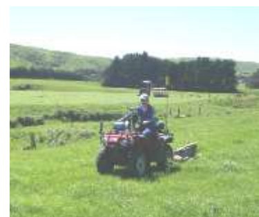
Figure 2 Conducting EM38 soil survey
