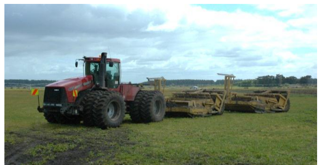
Precision levelling using high accuracy GPS
