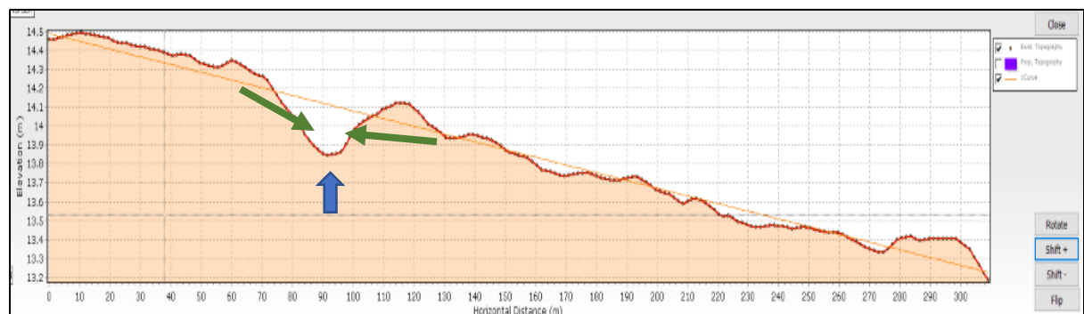
Figure 6. Row Elevation Profile: Cut and Fill Option 1
