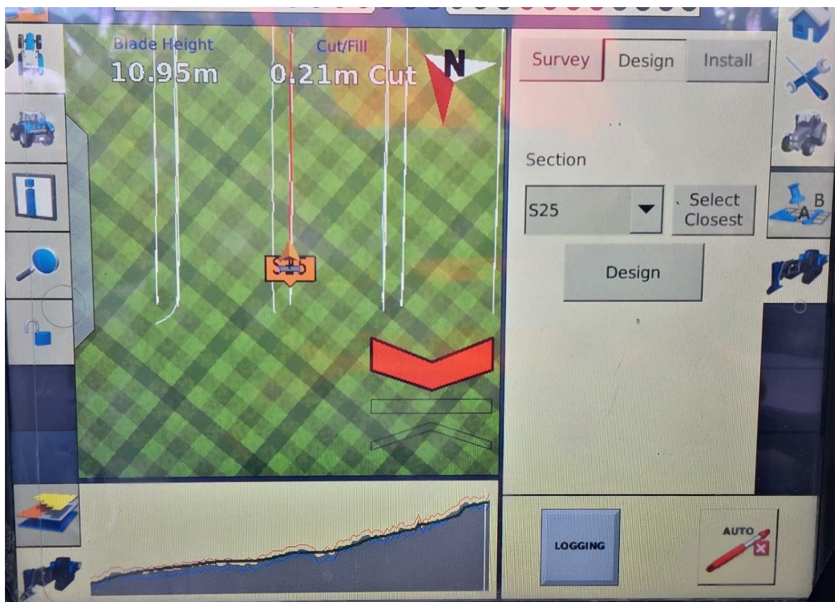
Figure 10. FMX screen post survey showing surveyed sections (lines) and the resolved profile after design selection.
