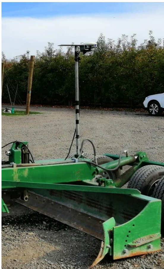
Figure 6. Antenna pole mounted above leveller blade
