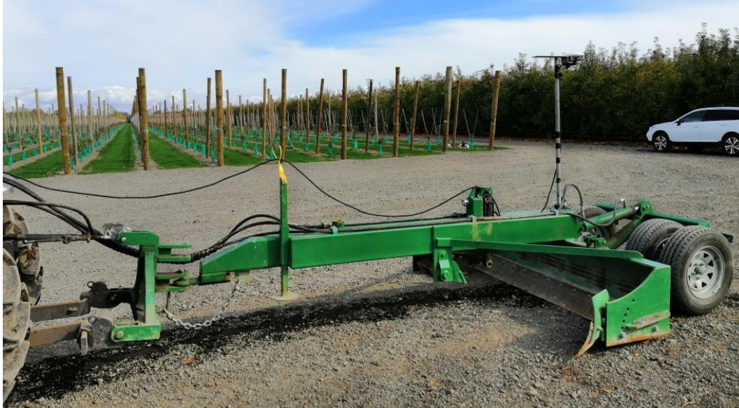
Figure 6. Gene Williams' Land Shaper connected to three-point linkage raw-bar
