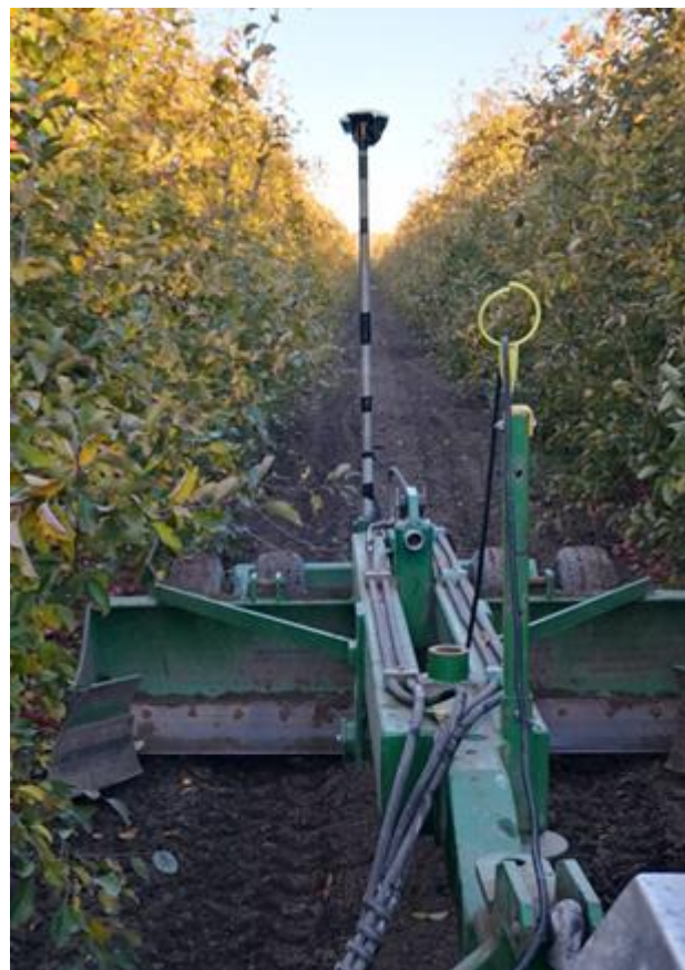
Figure 7. Keep equipment mounted centrally and protected from branches. Keep antenna high to minimise GPS signal blocking
