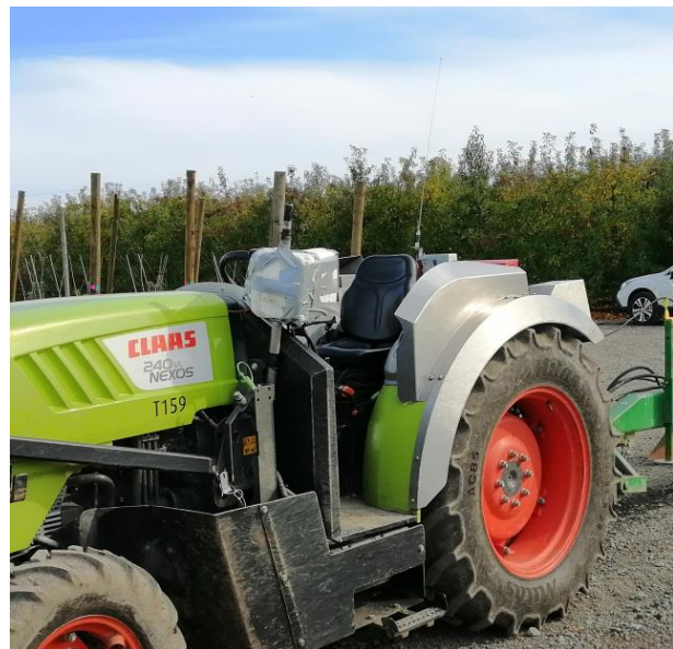
Figure 5. Tractor with mounted FMX protected by Shield, RTK digital radio mounted with aerial behind driver's seat
