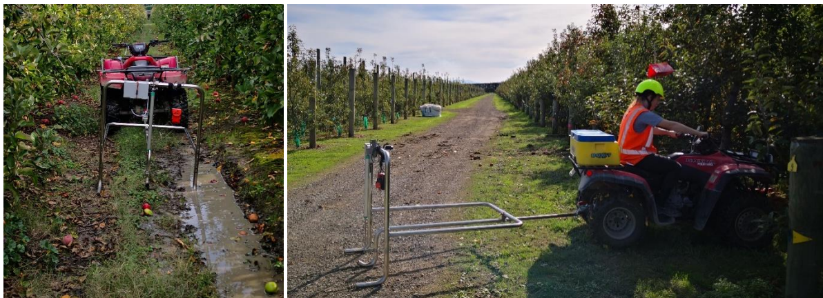
Figure 14: Sled design to measure rut depth, measuring the difference in height between the bottom of the wheel tracks and the centre of the inter-row.
