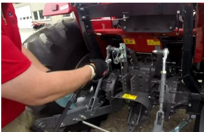
Figure 7 Connect hydraulic hoses to tractor remote hydraulic couplers
