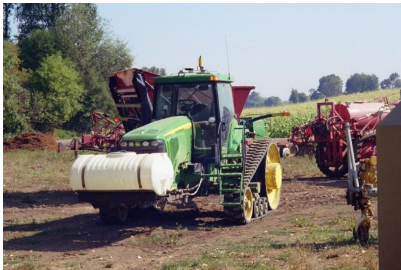
Fig 1. Tracked John Deere – narrow track width, fert tank on front, GPS equipment on roof
