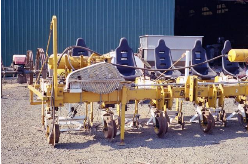
Fig 12. Mechanical weeder for squash and pumpkins
