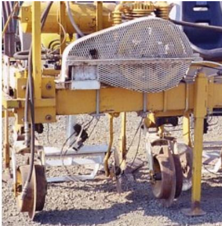
Fig 13. Detail of v-shape inter-row tine, discs, and raisable in-row weeding blade
