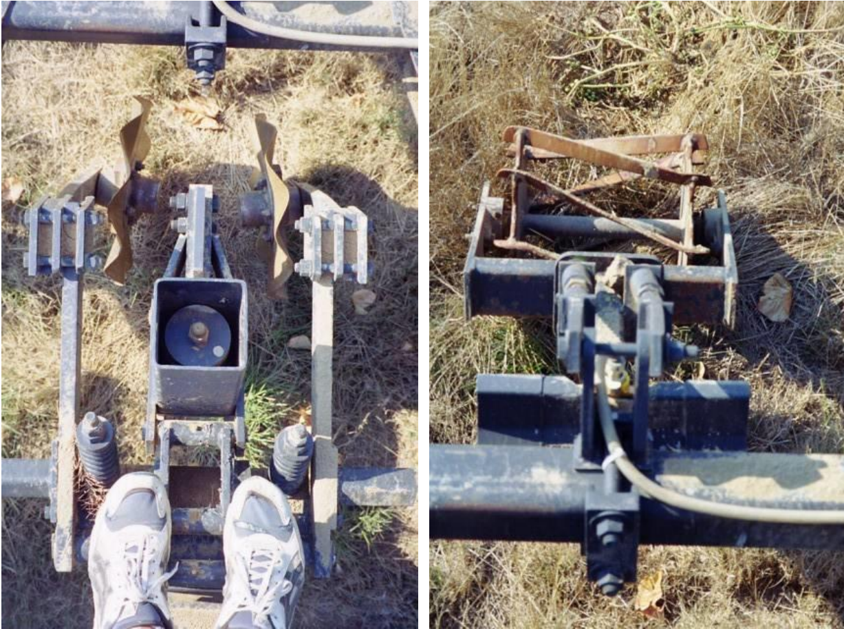
Figs 4&5. Primary cultivator for strip tillage showing disc arrangement and cage roller with fert nozzle
