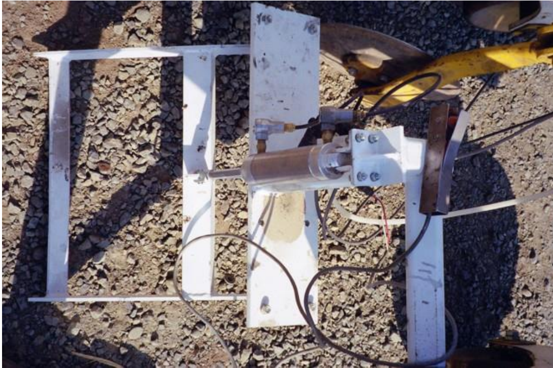
Fig 14. Detail of in-row weeding blade, lifting ram and trigger unit
