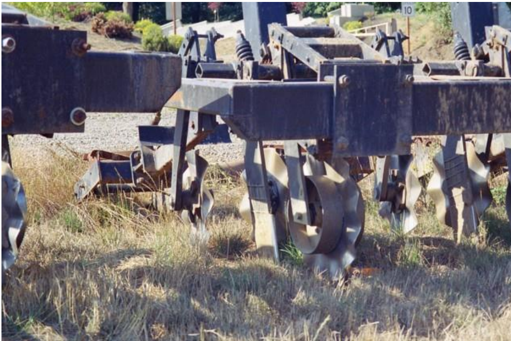
Fig 3. Primary cultivator for strip tillage showing disc arrangement and heavy mole knife
