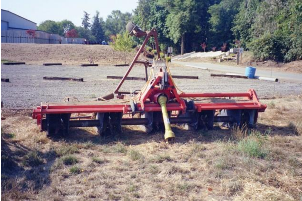
Fig 6. Secondary cultivator for strip tillage showing 5 shrouded rows of blades
