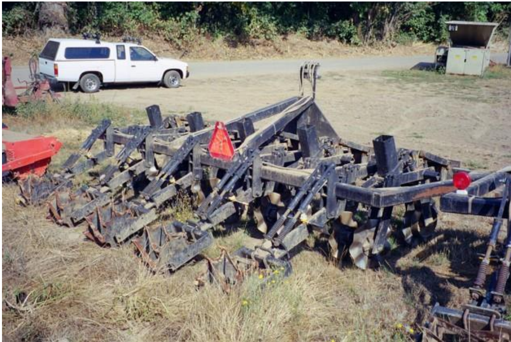
Fig 2. Primary cultivator for strip tillage showing disc arrangement and rear cage rollers
