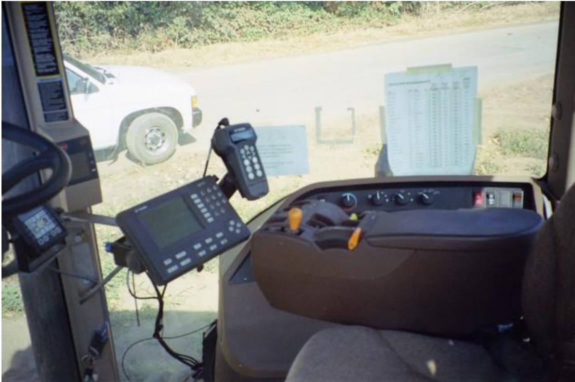
Fig 11. Precision ag screens in tractor cab, steering wheel folded away
