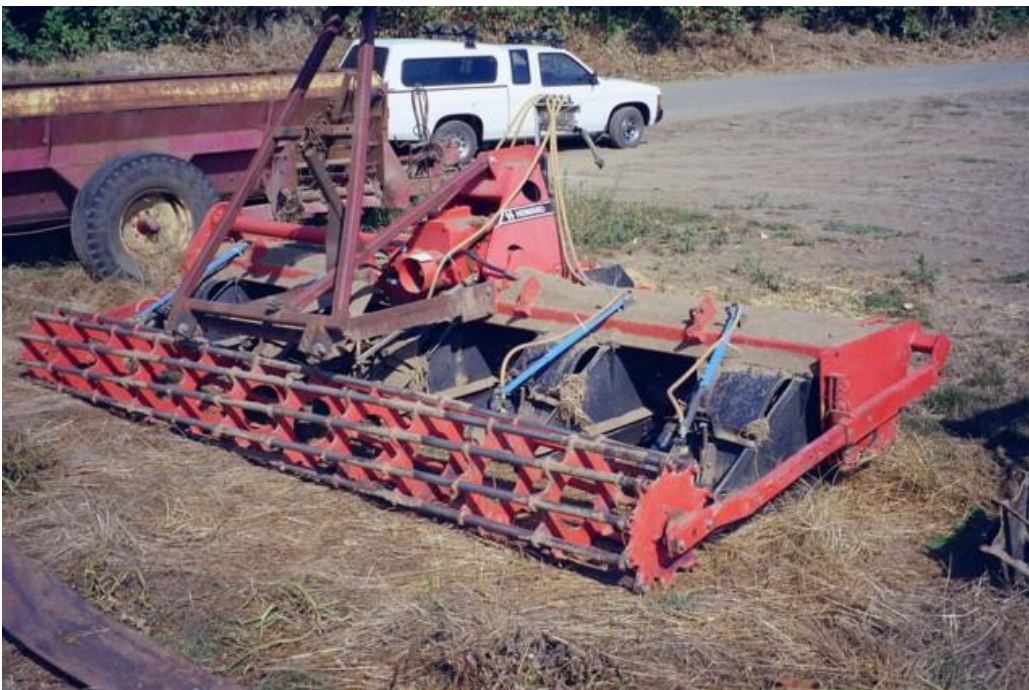
Fig 7. Secondary cultivator for strip tillage showing full width rear roller and rubber shields
