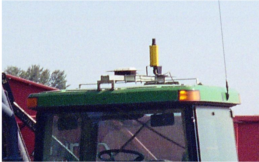
Fig 10. RTK GPS equipment mounted on tractor roof
