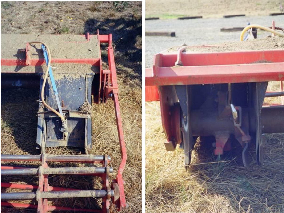
Figs 8&9. Secondary cultivator showing shields, fert nozzle & straight shrouded blades
