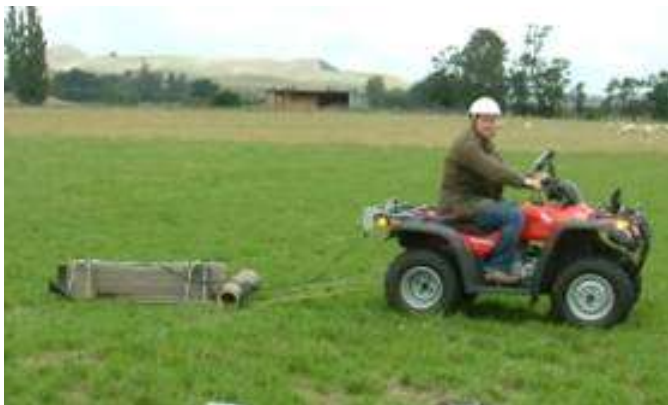
Figure 8 EM38 Soil scanner mapping soil variability, enabling detailed soil water holding maps to be prepared
