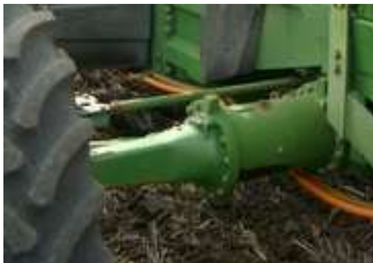
Figure 6 Axle extension to widen front track to 3 metres
