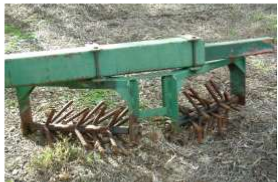
Figure 11 Prongs pull soil into wheel tracks after rutting has occurred
