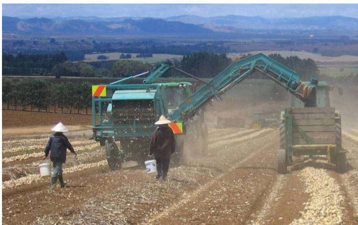
Figure 1 Harvester and trailer making use of permanent tracks.
