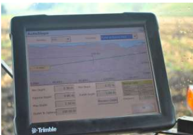
Figure 2 In-tractor computer console that calculates drain depth and controls laying operation
