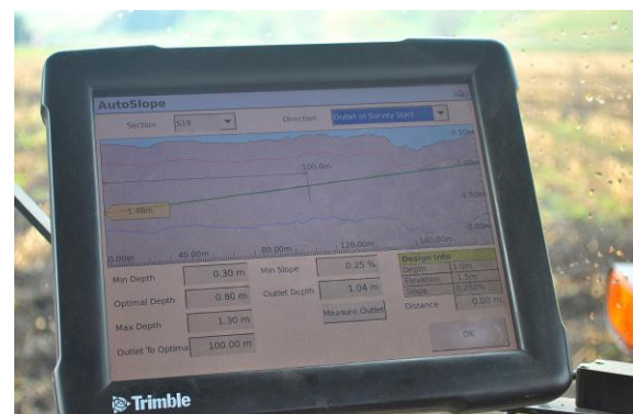
The console screen – gradient determined from GPS data and design rules
