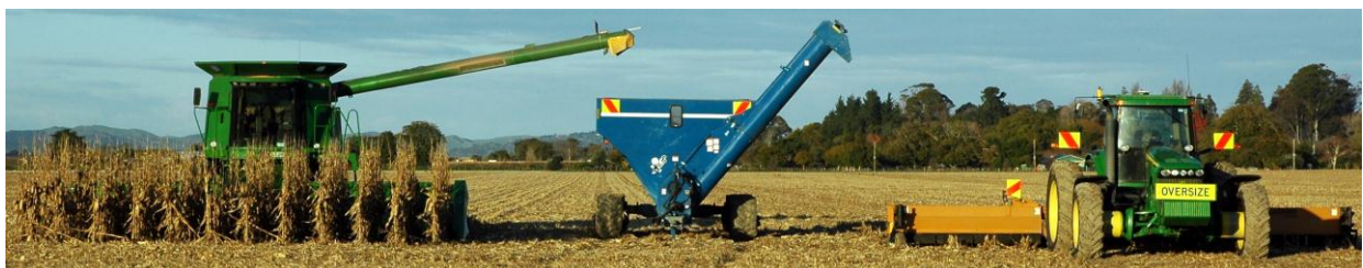
Twelve rows of matching equipment and GPS guidance means better soils, less fuel and less time in the tractor
